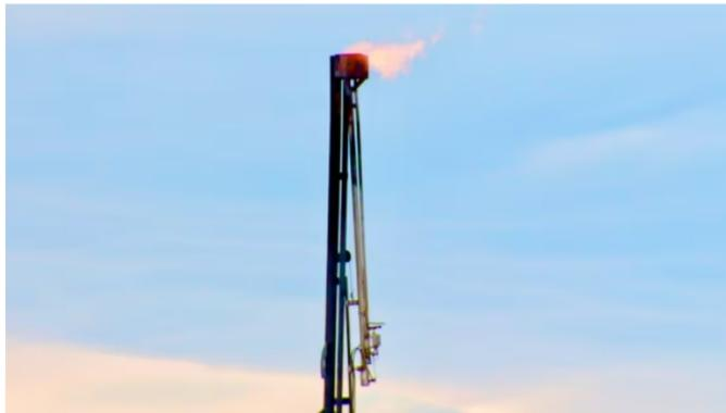
Oil producers use flaring to burn methane gases, rather than release them directly into the atmosphere. Venting and flaring accounts for about 42 per cent of emissions in Saskatchewan, significantly higher than in Alberta or B.C. (Kyle Bakx/CBC)
